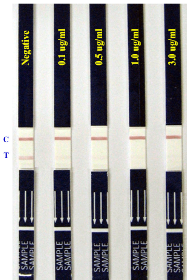
Fig. 7. IC strip test results at NVP concentrations of 0, 0.1, 0.5, 1.0 and 3.0 \mu\text{g/ml} in PBS pH 7.4. C, control line; T, test line.
